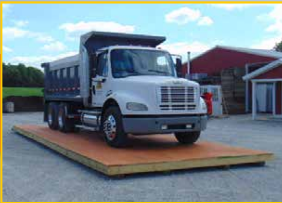
Testing the Double Super Tuff floor with a 20,400 lb. truck.
